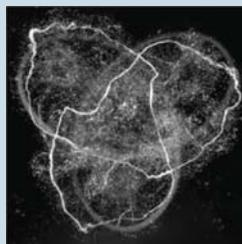
use a 3D printer to fashion hydrofoils whose topologies correspond to those desired of the vortices. One such hydrofoil, when placed in a water tank and given a swift tug, shed the trefoil vortex knot pictured here. (A video is available online.) Light-scattering microbubbles, which tend to get trapped along the vortex lines, provided a convenient
